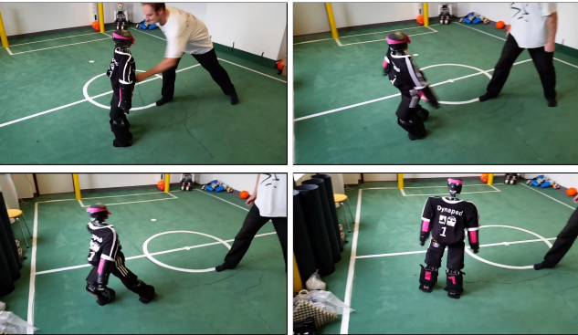
Fig. 1 Push recovery with bipedal robot Dynaped.
